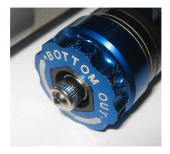
The nitrogen chamber bottom-out adjuster on the the DHX 5.0
