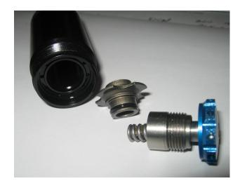
Propedal Valve, compensator spring and Propedal adjuster mechanism
