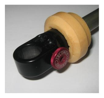
Once your sag is set properly the rebound adjuster can be set for the ride conditions, standard position is about 8 clicks counterclockwise out from full slow. Turn out 1 click to speed up rebound, this will make it absorb small close together bumps easier. Turn in 1 click to slow up rebound when absorbing big bumps to prevent kicking up. Repeat click at a time until desired results are achieved. Faster rebound is more desirable when trying to achieve plusher setting
