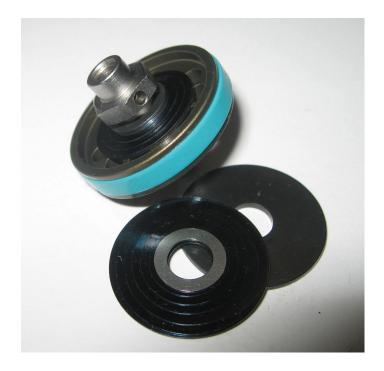
The removal of the Propedal and replacement with the SSD compression adjuster system now allows the main piston to be revalved for speed sensitive valving shims according to the linkage progression, rider ability and type of terrain.
