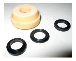
AVA Advantage Shape Factor Bottom-Out Bumper, HardCoat Friendly Dust Scraper, water and mud seal, and Viton Low friction Oil Seal An Improved shape factor anti-bottoming MX-style urethane bumper has been installed.
