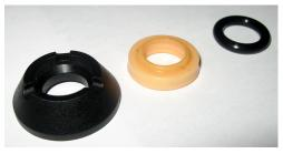
Stock DHX Bumper, Dust Seal and Oil Seal
